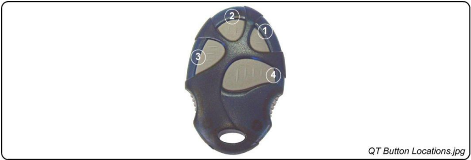
Figure 1: Button Configuration for ImproX (QT) Quad Transmitter Programmed in “Dynamic Code Transmission Mode”
