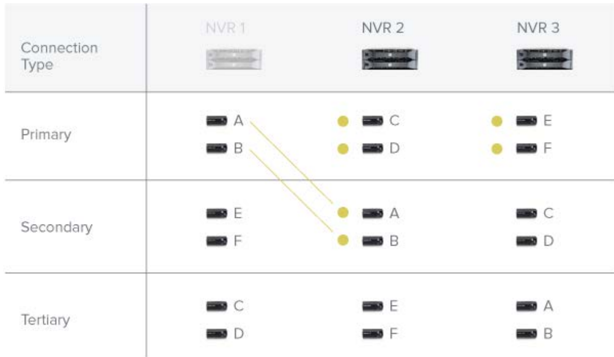
Figure B. NVR 1 fails
