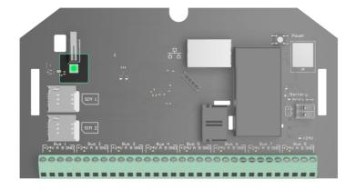
Depending on the state of communication between the control panel and the Ajax Cloud server, the Hub Hybrid LED indicator lights up in three colours: white, red, or green.
