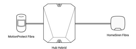
Hub Hybrid is a hybrid control panel of the Ajax security system. It controls the operation of the entire system and connected devices.
