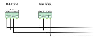
+24V — power supply input A, B — signal terminals GND — ground
