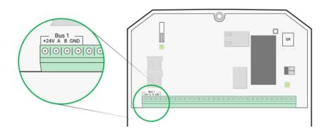
+24V — power supply input A, B — signal terminals GND — ground
