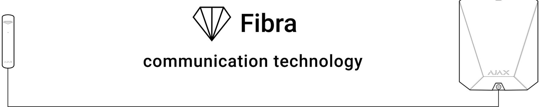
**Fibra** is a **two-way wired protocol**, ensuring fast and secure communication between hubs and devices. Based on a **bus connection method**, Fibra delivers instant data-rich alarms: security companies and users know which device was triggered, when and where it happened.
