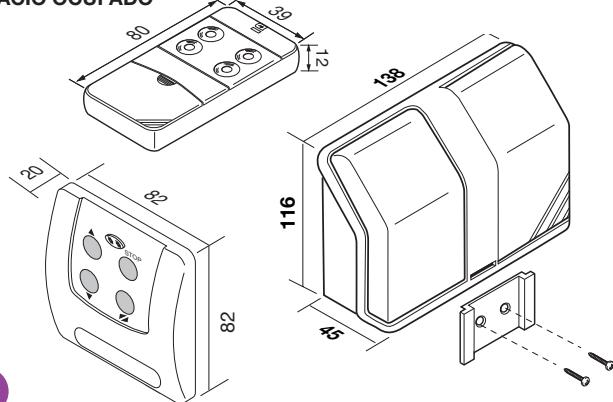
**RICEVITORE CON CONTENITORE - ENCASED RECEIVERS - RÉCEPTEUR AVEC BOÎtier - AUSSENEMPFÄNGER - RECEPTOR CON CONTENEDOR**
