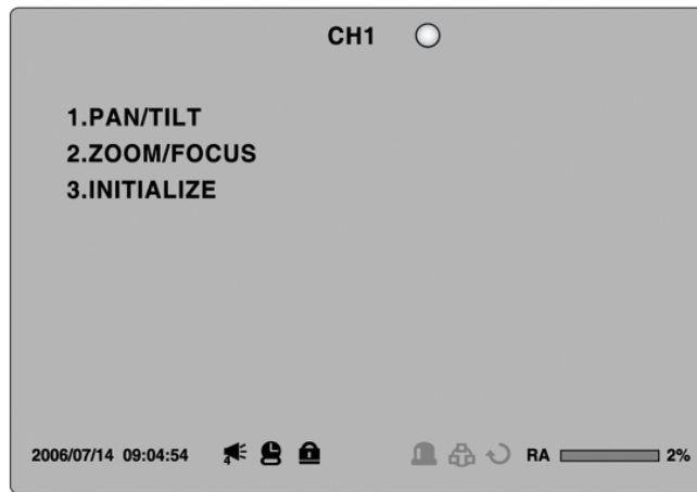
Figure 6.1.1. PTZ Control Screen
