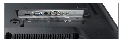
Video versatility, including VGA, HDMI, S-Video and BNC In/Out
