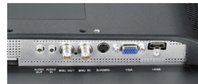
Video versatility, including VGA, HDMI, S-Video and BNC In/Out
