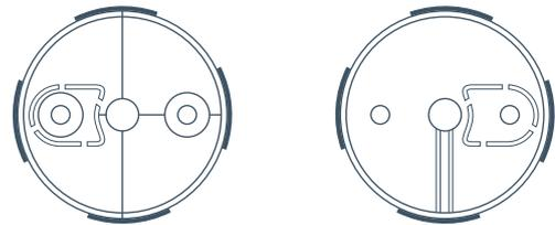
PICTURE 2. SmartBracket fastening panel
