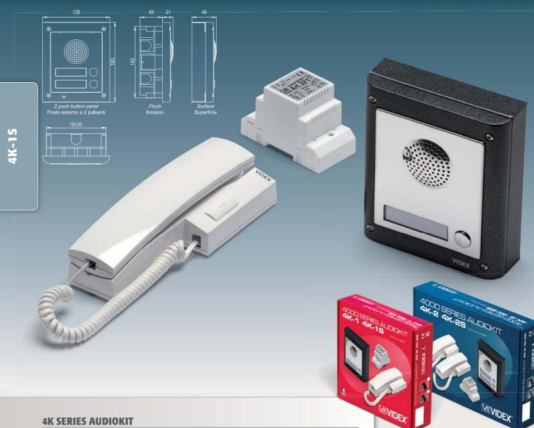
The 4000 Series audio door entry kits benefit from advanced features such as electronic call tone generation and lock release relay included within the door panel. This reduces the cable requirements between the handset(s) and the door panel to only 4 ("3+1") connections. For this reason larger cable distances using small cores sizes can be achieved between door panel and telephones.
