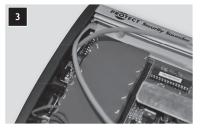
Cables shown entering the Sounder through thesse cable access holes.
