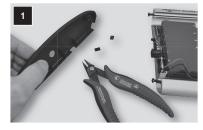
Cable access through the plastic endcaps i possible. Simply cut the prepared blankets using a sharp plier.
